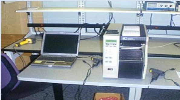
Lab 6- An RFID Smart Label Printer will be used to print Gen-2 labels
