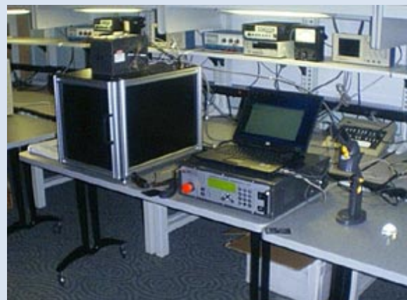
YAG laser etching equipment used to etch UID data plates
